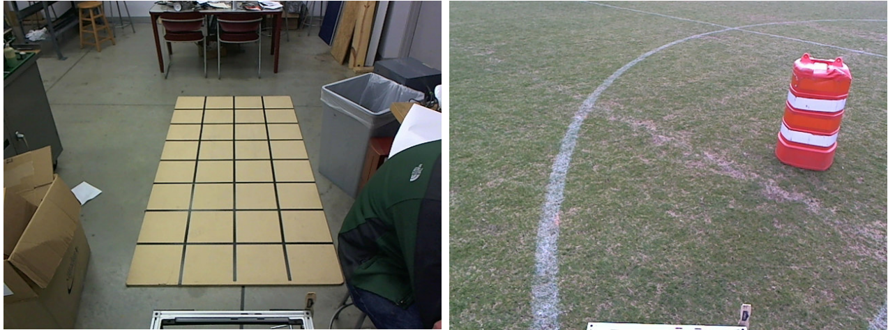
Figure 5.6: The figure on the left shows the method used for calibrating the camera. The figure on the right shows a snapshot of the webcam during the test runs.
