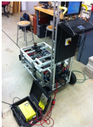
Figure 4.2: This figure shows the external battery charger case when removed from the robot unit (left) and when attached to the robot to provide battery charge (right).
