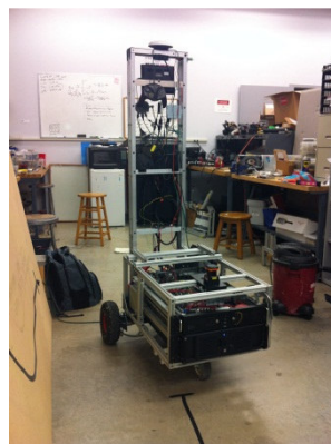
Figure 3.1: The figure on the left shows the original design frame of the robot with four wheels and three server rack cases. The figure on the right shows the actual frame of the robot with a castor wheel in place and two server racks.
