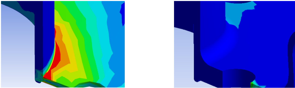
Figure 3.2: Stresses at joint for original hub (left) and redesign (right).
